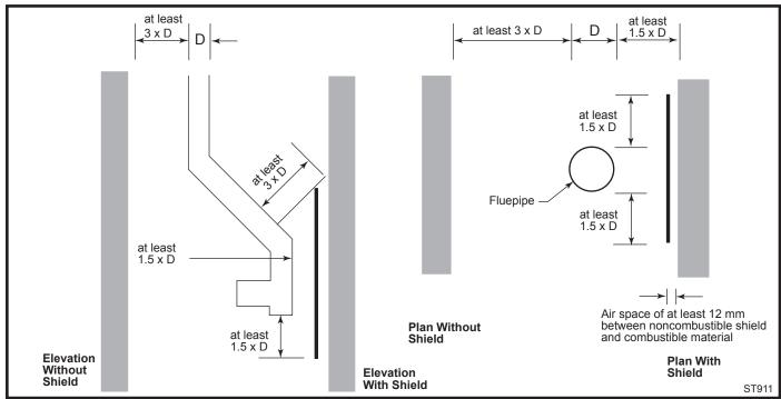
Fig. 12 Connecting fluepipe clearances.
